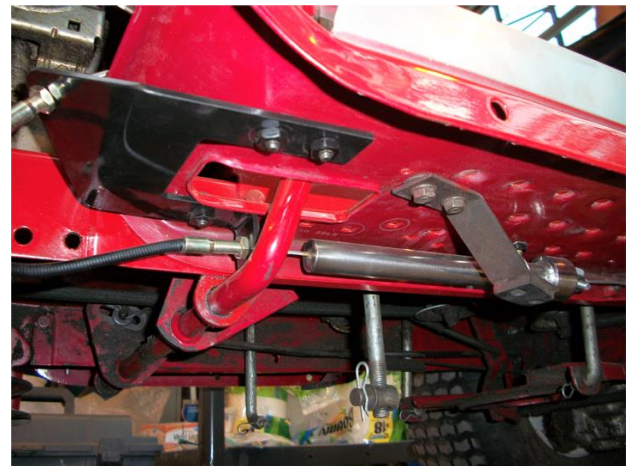
Fig. 19.16. Tensioner unit installed under floor plate.
