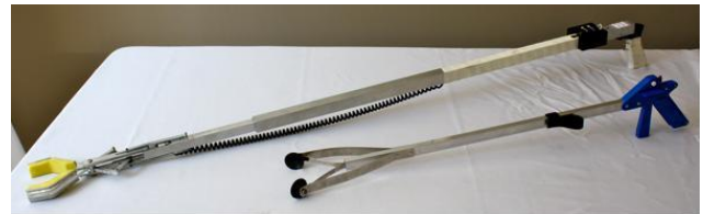
Fig. 19.5. Developed prototype (to the left) next to commercially available Easy Reacher (right).
